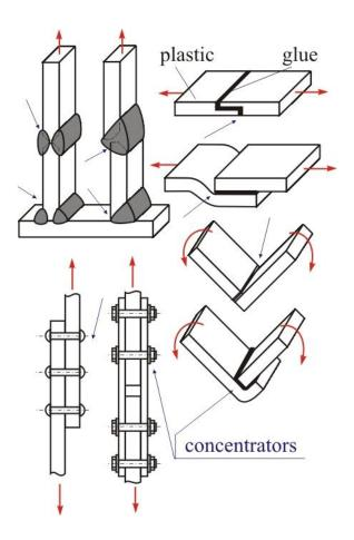
Glued joints also show stress concentration due to the non-uniformity of elastic properties and the change of geometry. Rivets and bolts are inserted into holes that are stress concentrators. Force lines must bend around the joints, which causes concentrations of the force lines at the joint.
