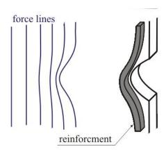
For proper design, the zones of transition from rigid to more flexible components should not include sharp corners, sharp bends, thin flexible layers, and so on.
