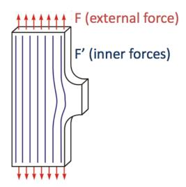
To describe the inner forces in a section of the structure we use stress defined as the force divided by the cross-sectional area. Stress corresponds to the force acting on a unit of area (square millimeter, square inch, square meter, etc.). A smaller cross-sectional area creates a larger amount of stress under the same external force.
