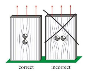
2) Enlarging the radius of curvature in a notch,
