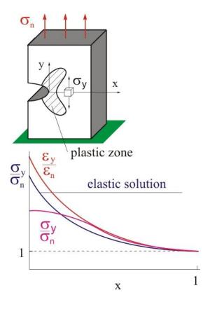
The opposite occurs with strains. A strain in the notch tip is larger than that in the elastic body. In real materials, stresses in the crack (the sharpest concentrator) will not reach infinity due to plastic or nonlinear deformation.
