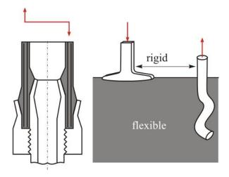
A stress concentration will occur near a broken rigid fiber in a flexible matrix. Delaminating fibers from the matrix will help "smooth" the redistribution of force lines.
