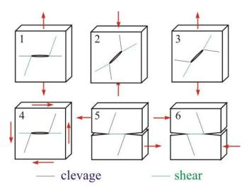
The main mechanism of fatigue crack initiation is local plastic deformation (e.g., on the neighborhood of a stress concentrator). The growth of fatigue cracks is higher if the maximum stress is greater than the limit of elasticity for the material. In this case, the time for crack initiation and growth is short.
