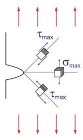
There is three-dimensional state of stress in the notch. The complex stress state is only in the small area near the tip of the notch. In the other points of the structure, there are tensile stresses only or no stresses at all ("dark corners").
