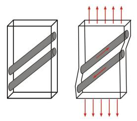
A plate is reinforced with a concentrator according to the distribution of the force line. An effective method is to place reinforcement bars along the main force line.
