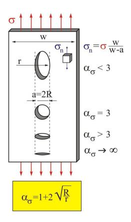
The formula shown here is valid for an elliptical hole in an infinite plate. Only in theory does the stress concentration factor tend towards infinity for a crack (radius of curvature is equal to 0).
