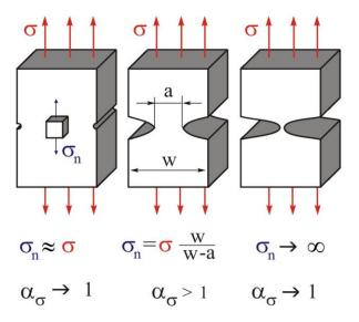
Elliptical holes can be problematic if the larger axis is perpendicular to the applied tension. In this case, the width of the "obstacles" on the force line path is large and the radius of curvature in the notch tip is small.
