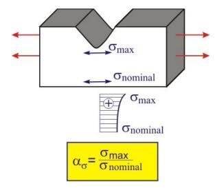
The authors of the theory of elasticity proved that tensile stress near a hole in a wide plate is three times higher than nominal stress. This means that the stress concentration factor is equal to 3 in this case.
