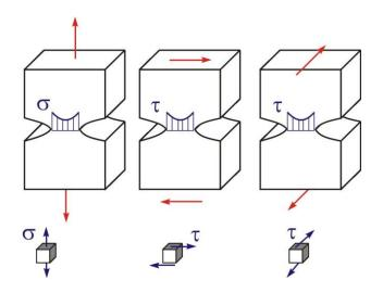
For biaxial tension or more complicated loads, the principle of superposition is applied.
