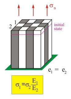
Rigid fibers define the deformed shape of composite materials. The material in a more flexible matrix has larger shear deformations.
