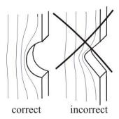
3) Removing stress concentrators from regions of tensile stress,
