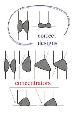
At the edges of glued surfaces and welds, there is an increase in shear stresses. The main reason for this increase is the difference in the rigidities of the connected plates at the ends.
