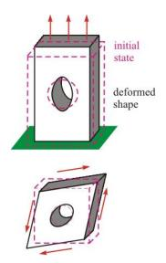
Usually, nominal stress is defined as the average stress in a cross-section. Consider the three situations to the right. In the last case, the stress is very high due to the large amount of nominal stress. The stress concentration for the third scheme is lower.
