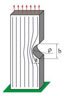
Theoretically, if the radius tends towards 0 (sharp crack), the stress concentration factor tends towards infinity. That conclusion is correct only for an ideal elastic body. In real structures, the stress concentration factor is finite due to plasticity and microstructural changes. Thus, the stress concentration factor increases as the radius of curvature in the notch tip decreases.
