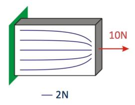
For any state of stress, it is possible to determine the direction of the maximum tensile stress. This stress is called the main stress. Force lines are drawn by the integration of the main stresses. Mathematical methods are used to draw force lines. We use a few simple rules to present force lines:
