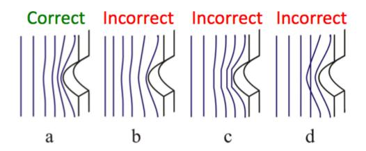
Both tensile and compressive force lines can be used in the analysis. Usually, compressive lines are perpendicular to tensile lines.
