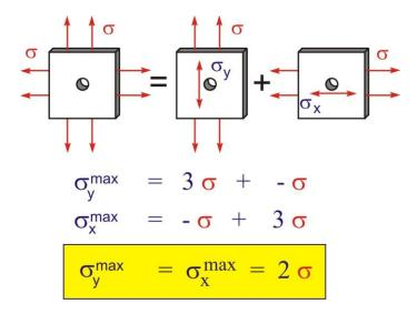
For example, biaxial tension is the superposition of two applications of tension and this has twice the maximum stress as nominal stress.
