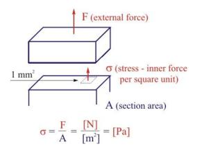
As a result, compressive and shear forces also cause compressive and shear stresses. As a rule in complex structures, tensile stress results in compressive stress in the perpendicular direction.
