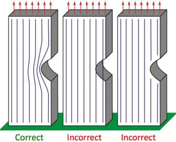
Force lines are distributed uniformly for tension. Their density is higher at the edge of a beam under bending.
